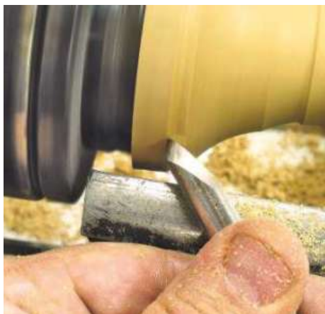
▲ Pic.28 Put the sanded lid to one side and finish turning the base section. When working up near the chuck make sure you start the cut like this to stop the tool skating along the wood into the chuck
